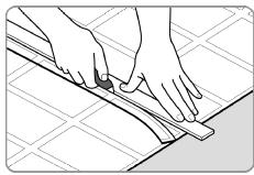
gap. Cut each side before trimming the linoleum in place so that you have enough material left to re-cut one or both seam edges, if necessary.
