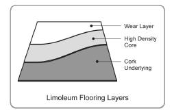
Floating linoleum goes through all the same manufacturing process as linoleum sheets and tiles. The linoleum is then mounted on HDF or other type of base board and covered with a thick wear layer on top. Additionally, some floating linoleum has pre-attached cork or foam underlayments.
